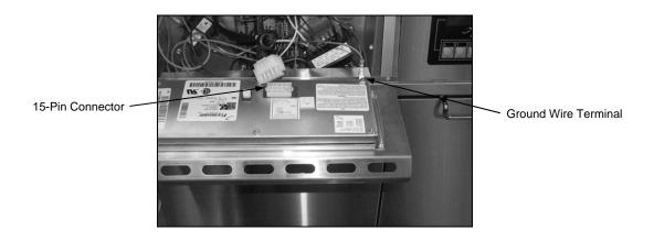
5. Remove the controller from the control panel assembly and install the replacement controller. Reinstall the control panel assembly by reversing Steps 1 and 2.
